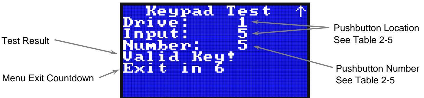
**Figure 2-54, Display – Keypad Test Screen**
