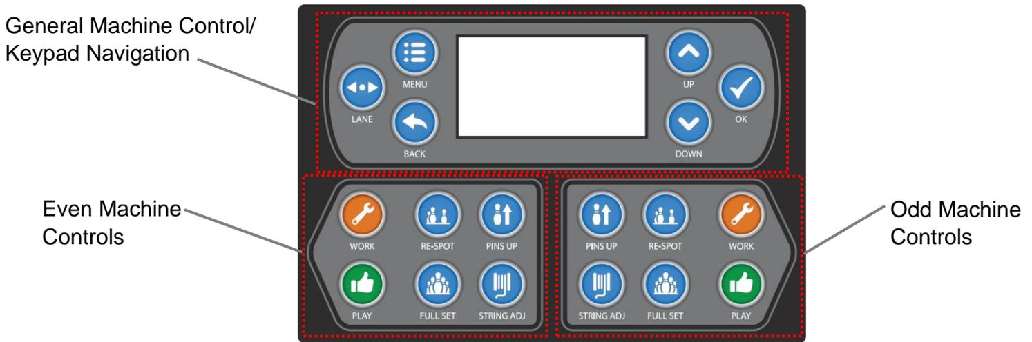
Figure 2-49, System Controller Keypad
