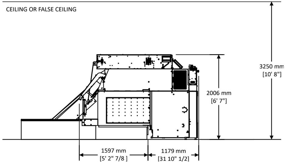
**SIDE VIEW WITH VIRTUAL CURTAIN WALL** of a pinspotter with the Heights and Widths required:
