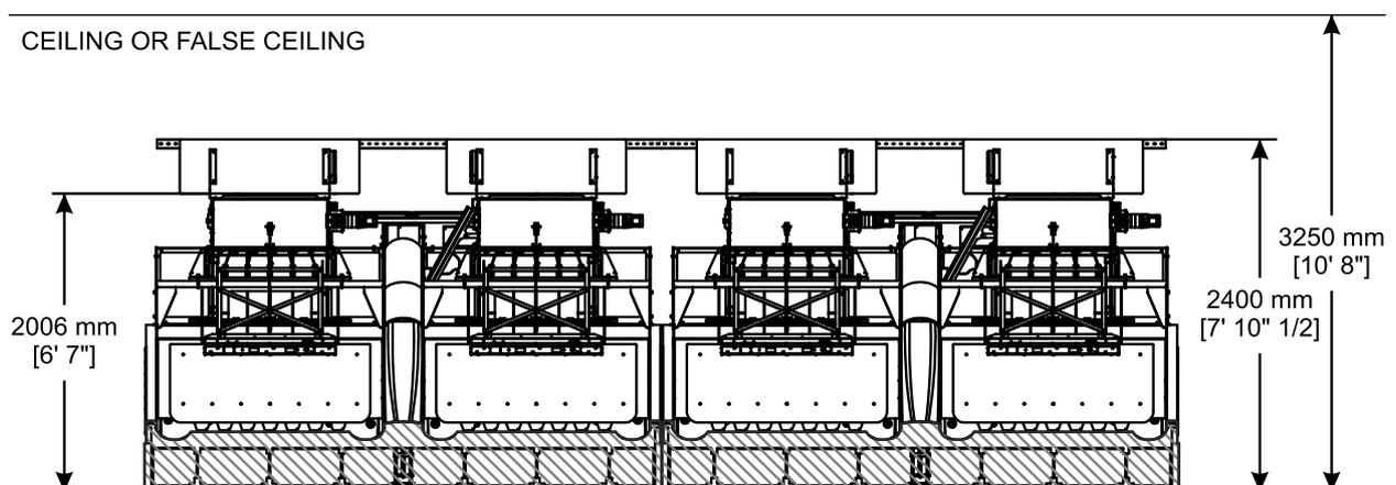
**SIDE VIEW WITHOUT VIRTUAL CURTAIN WALL** of a pinspotter with the Heights and Widths required.
