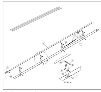
610049075-X - Kit consists of two 5' bumper rail sections with U-brackets and screws to couple them into one 10' replacement rail.
